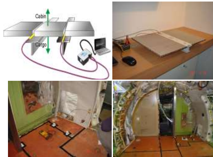
Fig.1 The applicability of the system was shown in a relevant lab-environment, and the sensor is in the meanwhile implemented in an operational airliner (Boeing 737). The sensor network will provide first data on the presence of corrosive liquids in a relevant environment.
