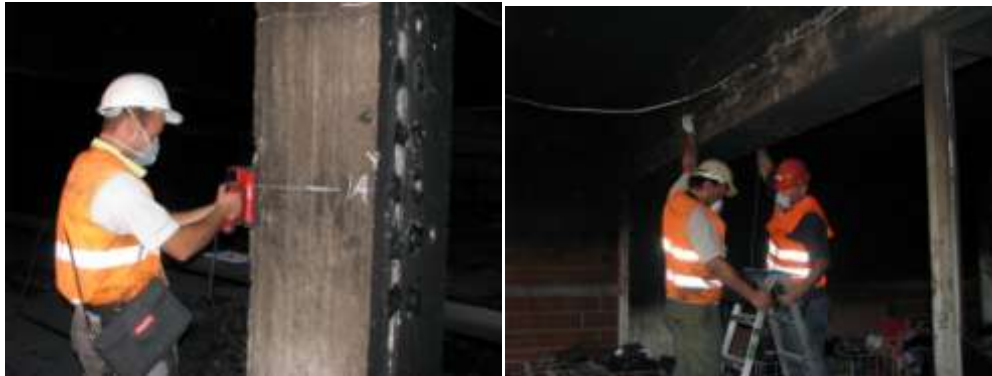
Fig. 1: Direct ultrasound pulse velocity measurement (left) and reinforcement cover depth measurement (right)
