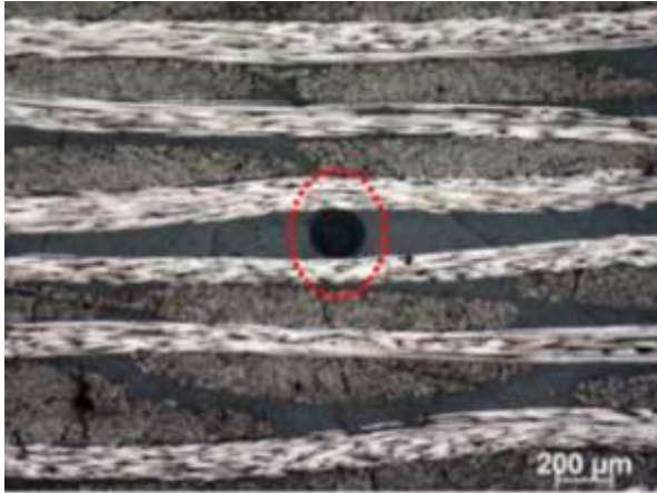
Fig.1: Embedded optical fibre sensor in satin weave composite
