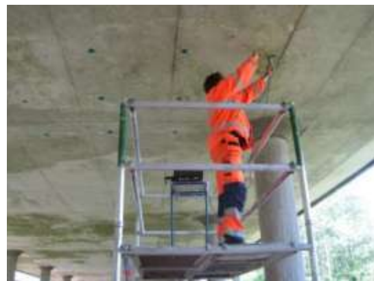
Figure 1. Impulse Response Testing on Evripos Bridge, Greece (left) and Impact-Echo, Demark (right)
