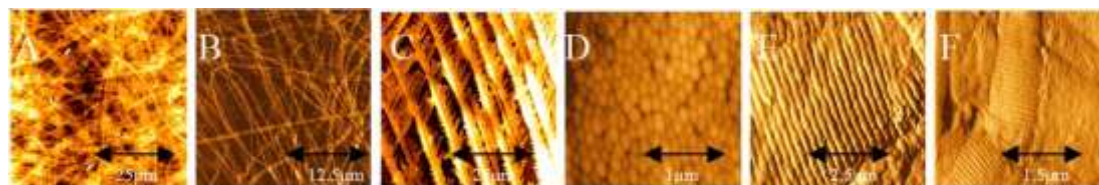
Fig. 1: AFM topographic images of collagen thin films and their substrates: Elongated fibers with random orientation on glass (A) and mica (B) with spin coating procedure. Oriented collagen fibers, formed by hydrodynamic flow of the collagen solution over the substrate (C), Polystyrene particle surface (D). The characteristic D-band of collagen fibers formed on polystyrene particle surface (E) and mica (F)
