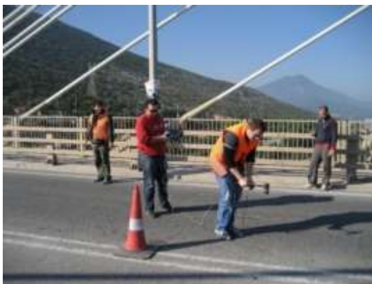
Figure 1. Impulse Response Testing on Evripos Bridge, Greece (left) and Impact-Echo, Demark (right)
